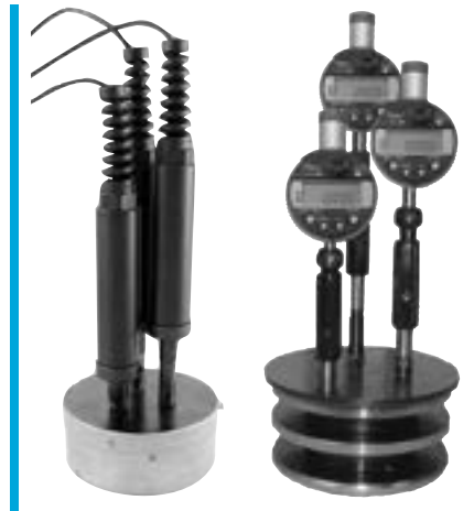
3 Ø's, Taper, out-of-round, TIR
