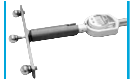
Model 136-210 custom design for diameters larger than 31.00". Special contacts and centering-base designed for measuring the I.D. of large bearing races.
