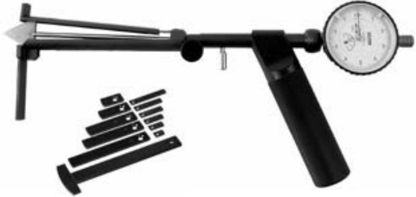
211-007 Probe body with 210-001 handle and various individual measuring contacts.
