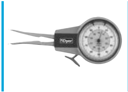
104 Series 104-102 Special Contact arms modified to enter 0.080" tube for 0.150" depth.
