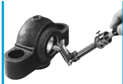
Contact point rotated 180° to enter small bore
