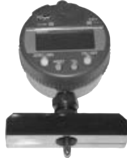
Special depth gage to measure dimple indentation on part surface. Gage's base modified to set correctly on part
