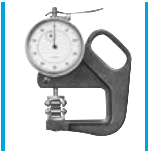
305-555 Thickness Gage, Roller Contacts Range: 0-0.2" Grad: 0.001" Width of roller = 0.34" Measuring force = 120 gm.
