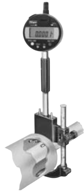
The gage will set flat against the part allowing the gaging to be electronic and non-tipping with no operator influence.
