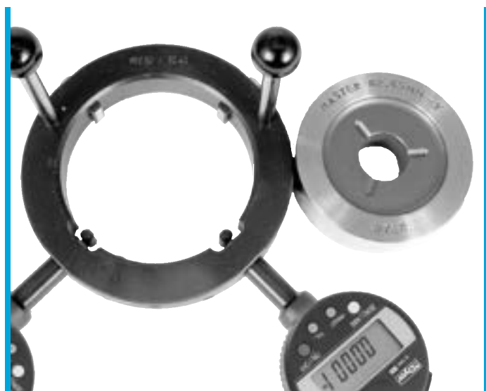
283 Special OD gage to measure splined part.
