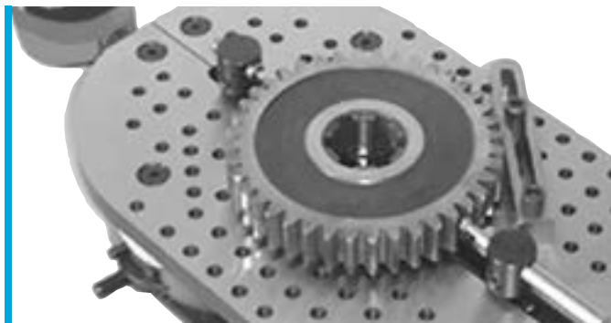
747 Series Measuring external pitch diameter using special size carbide balls and part stop
