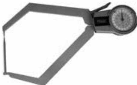
302 Special Measure bottom wall thickness of flower vase.
