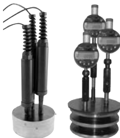
3 Ø's, Taper, out-of-round, TIR
