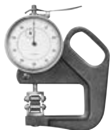
305-555 Thickness Gage, Roller Contacts Range: 0-0.2" Grad: 0.001" Width of roller = 0.34" Measuring force = 120 gm.
