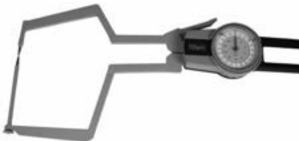
Measure bottom wall thickness of container.
